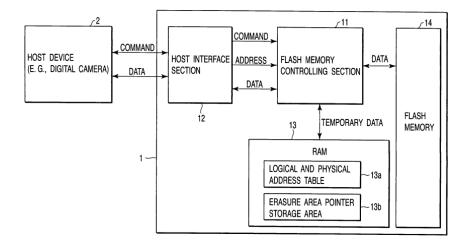
*Id.* col. 2 ll. 19–21, FIG. 1. In Figure 1, host device 2, such as a digital camera, is connected to memory card 1, which
