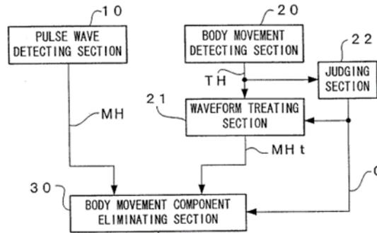
The device also includes body movement detecting section 20 and waveform treating section 21. *Id.* at 21:9–12. If no body movement is present, the operations of waveform treating section 21 and body movement component eliminating section 30 are suspended. *Id.* at 21:65–22:2. According to Amano, this suspension reduces the power consumption of the device. *Id.* at 22:4–6.
