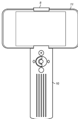
J.A. 43. Figure 3 shows the invention from another angle, without the handheld terminal but pointing out the slot sliding plate (9), which may be adjusted so the invention may hold differently sized mobile phones:
