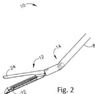
The articulation joint allows the shaft to articulate along two axes. Articulation cables couple the articulation joint to the tool mounting portion, such that the articulation joint may be operated by rotary motion from the robotic system. The '969 patent also contains tactile feedback sensors in the end effector.
