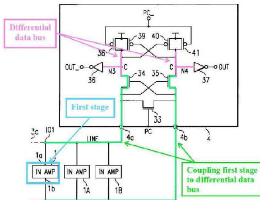
In the diagram, Samsung identified the differential data bus as the lines associated with nodes N3 and N4 (also labeled C), which connect the transistors 38–41 to the transistors 34 and 35 as well as to CMOS inverters 36 and 37. *See Sukegawa, col. 8, ll. 49–53.*
