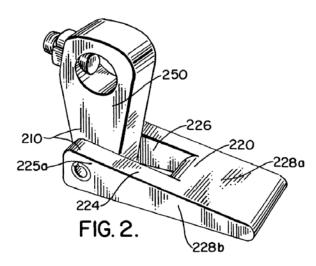
'871 Patent Figure 2. The "cam member" labeled 220, corresponds to SW1, and the "cam connector," labeled 250, corresponds to SW2.
