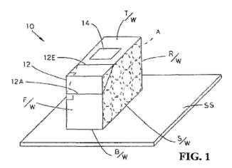
The closed form of the preferred embodiment has a scored or perforated line around the front top corner, which consists of a diagonal line across the two sidewalls connected with a line across the top and front walls. By removing the top front corner along the perforated lines, one gains access to the cans. The specification teaches
